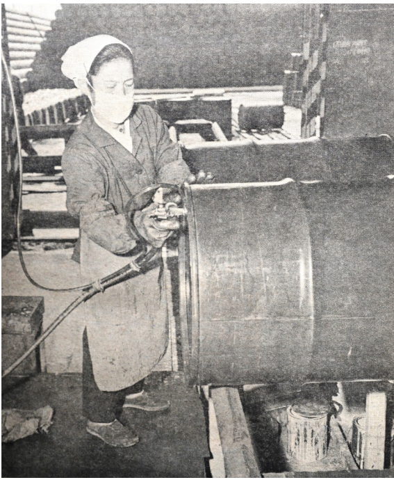
A Japanese employee at U.S. Army Petroleum Subdepot Tsurumi's drum reclamation plant in Yokohama sprays the inside of a 55-gallon drum with preservative oil to prevent corrosion in March 1967.
