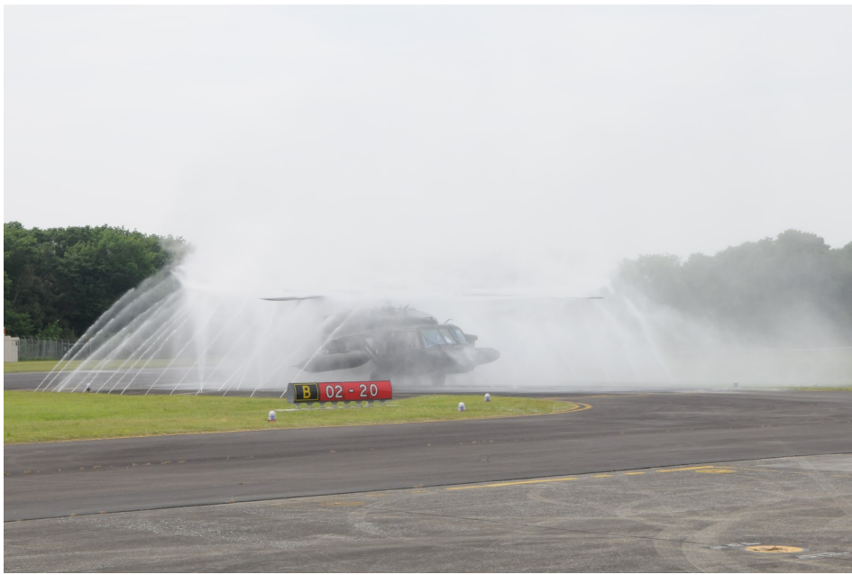
A UH-60L Black Hawk helicopter goes through a bath to remove salt from its airframe. U.S. Army Aviation Battalion-Japan aircrews completed deck landing training with the Japan Maritime Self-Defense Force ship JS Amagiri (DD-154), May 10, 2019, to maintain its periodic over water training requirements.
